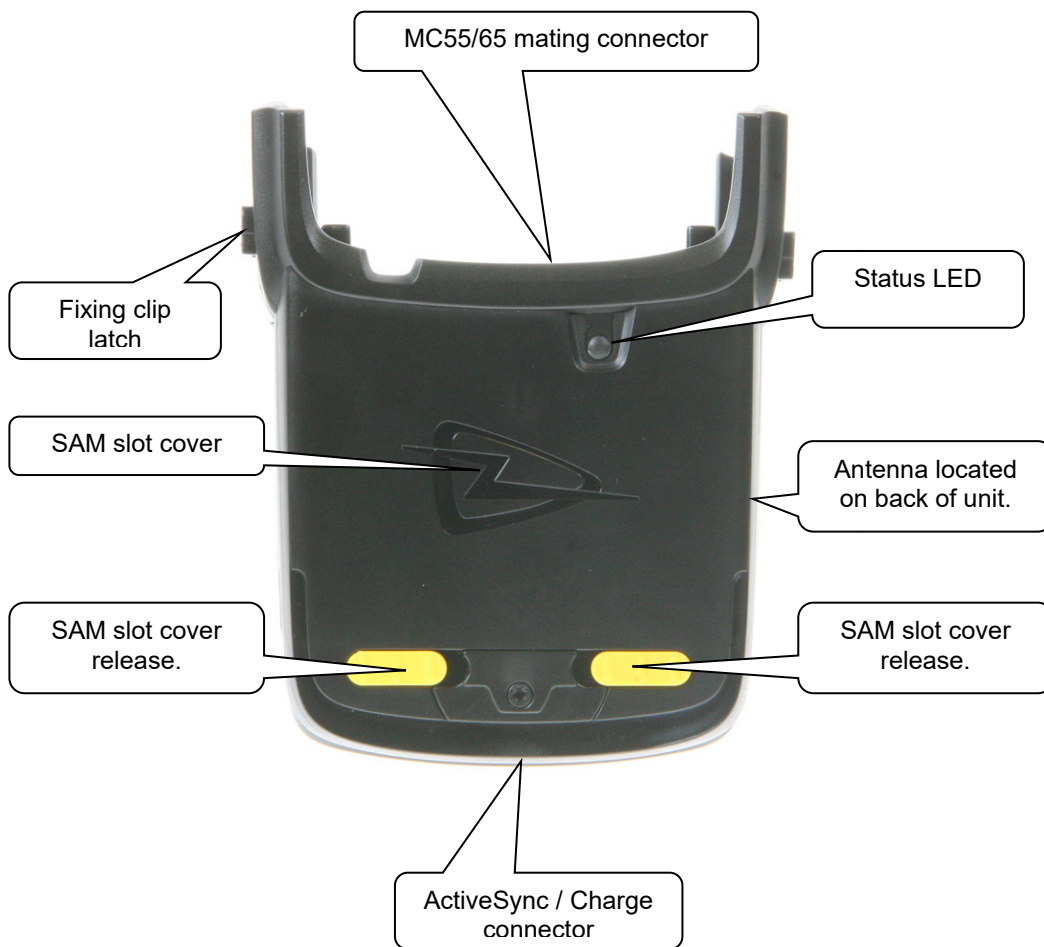
Figure 1: Parts of the 1117 HF Reader
